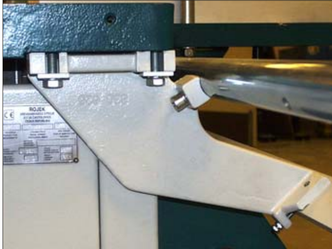
I-A Table support mounting bracket.
