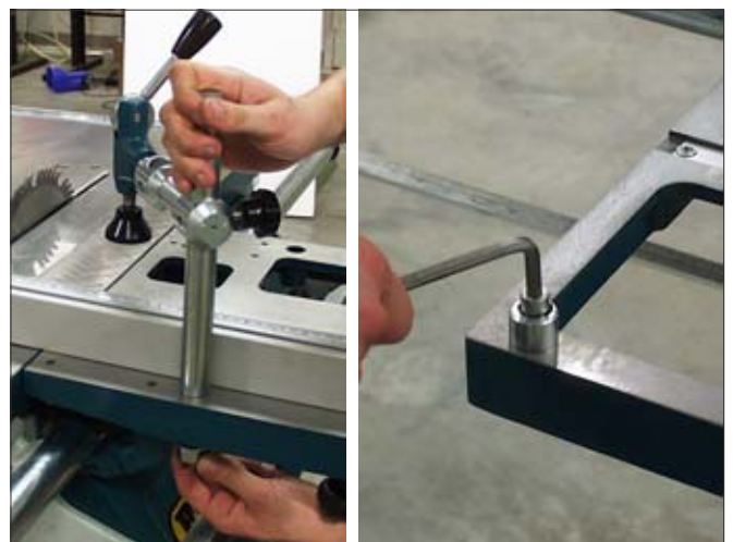
I-J Wood Clamp and Crosscut Fence 0° positive stop.
