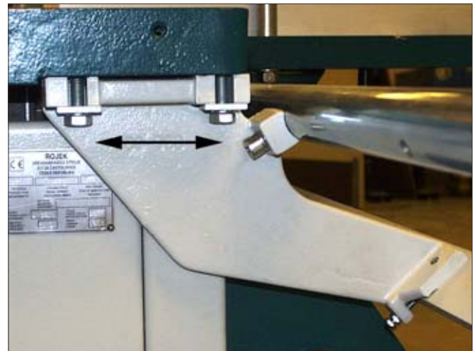
S-K Table support mounting bracket.
