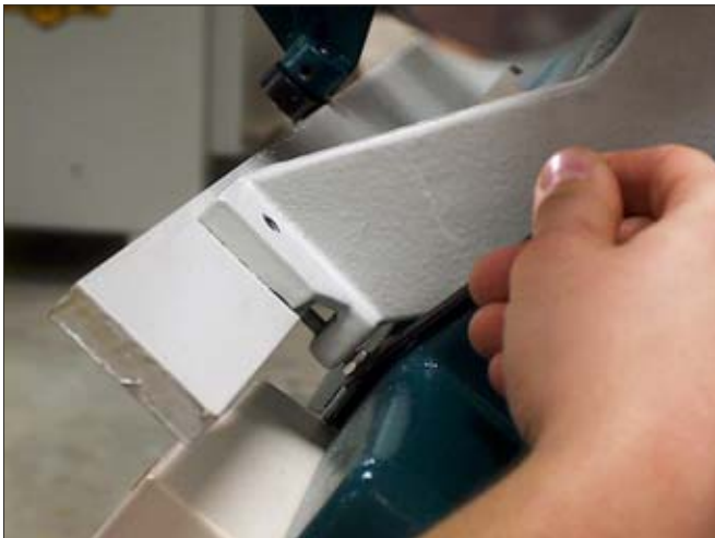
S-B Adjusting flat support bar height adjusting bolt.
