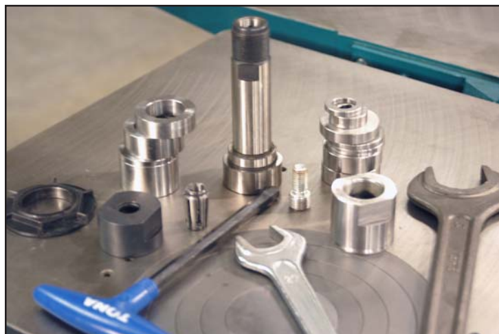
Components and tools for the 5/4" diameter router spindle. This is a special spindle with a shorter length for router use.
