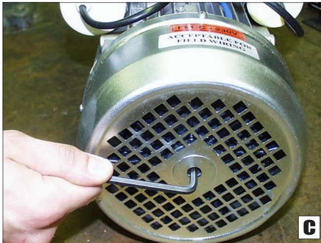
Adjusting the braking gap through the fan cover.
